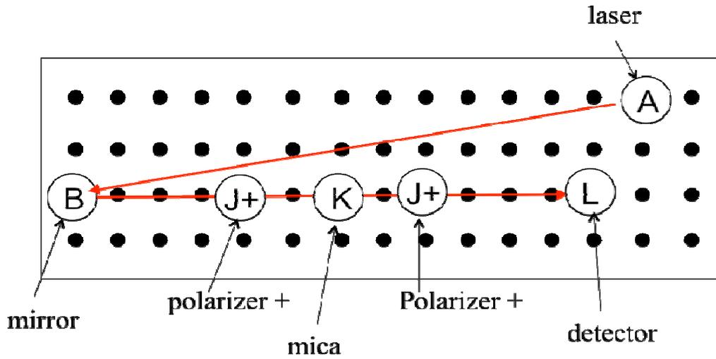
Task 2.1 b) Experimental setup for  $I_o$ . (0.5 points)
