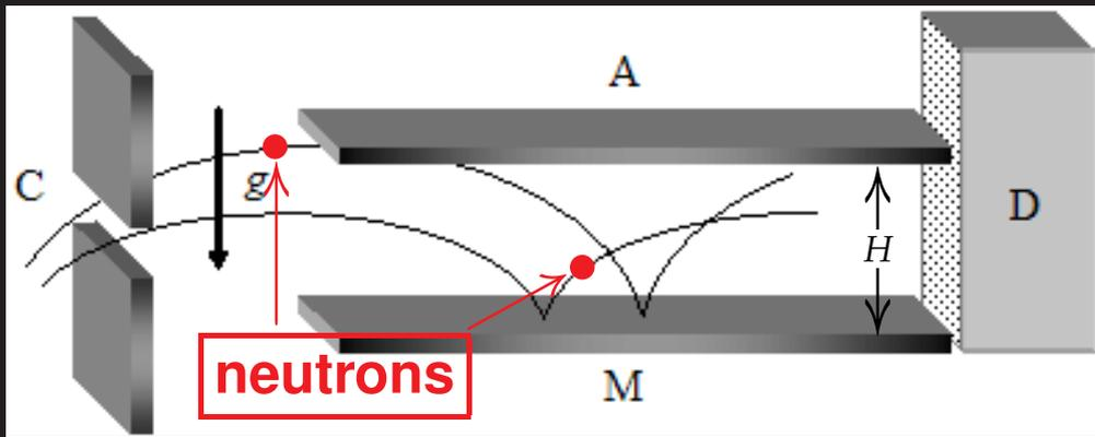
For neutrons ( $mv_z H \sim h$ ), the cavity behaves as an energy selector
