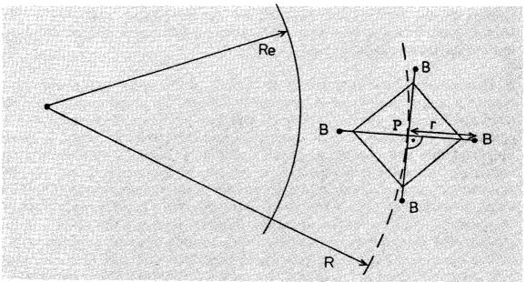
The link wires are included in the system in order to prevent oscillatory movement of the individual bodies B which would otherwise make the analysis of the movements extremely complicated. All the bodies B rotate around P at the same angular velocity, which is  $\omega$  with respect to the fixed stars. Thus, the satellite behaves as a rigid body.
