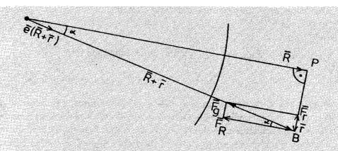
Figure 2: Analysis of the forces acting on body B in the sideways position. The angle  $\alpha$  is given by  $\tan \alpha = r/R$ . The tension is  $F_r = \sin \alpha F_g \approx \tan \alpha F_g = F_g r/R$ .
