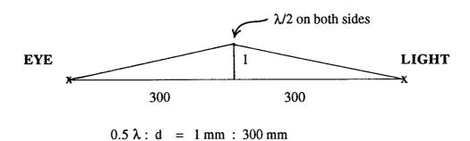
The middle wave length of visible light is 0.55 µm which gives 80 µm for the grid constant.
