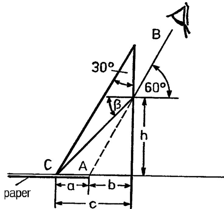
Place edge C of the prism on edge A of a sheet of paper and look along the prism hypotenuse at edge A so that your direction of sight B-A and the table surface form an angle of  $60^\circ$ . Then shift the prism over the edge of the paper into the position shown, such that prism edge C can be seen inside the prism collinear with edge A of the paper outside the prism. The direction of sight must not be changed while the prism is being displaced.
