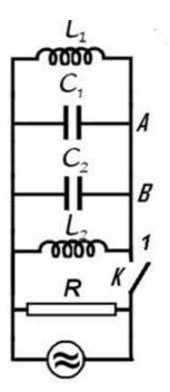
$i_{02}=0.2$  A  $L_1$  (the currents flow as in the figure); at the same moment, the potential difference on the capacitor with capacity  $C_1$  is  $u_0=40V$ :
