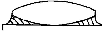
Because the refractive index of water is known in this case, one can evaluate the curvature radius through the formula above, where  $r_1 = -r$  and  $r_2 = \infty$  :
