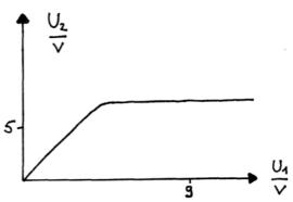
Comment: After exceeding a specific input voltage  $U_I$  the output voltage increases only a little, because with the alteration of  $U_I$  the current I increases (breakdown of the diode) and therefore also the voltage drop at the resistance.
