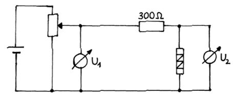
The graph of the function  $U_2 = f(U_1)$  has generally the same form for both directions of the current, but the absolute values are different. By requesting that the semiconductor element has to be placed in such a way, that the output voltage  $U_2$  is as high as possible, a backward direction should be used.
