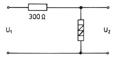
The input voltage  $U_1$  varies between 0 V and 9 V. The semiconductor element is to be placed in the circuit in such a manner, that  $U_2$  is as high as possible. Describe the entire circuit diagram in the protocol and discuss the results of the measurements.
