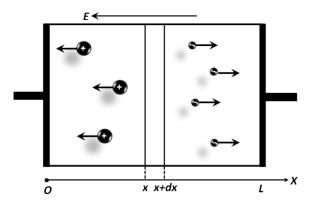
avalanche isexplained as follows. The electric field accelerates free electrons which acquire enough kinetic energy to ionize the atoms in the gas by hitting them. As a result the number of free electrons moving towards the anodesignificantly increases. This process is described by the Townsend coefficient  $\alpha$ , which characterizes an increase in the number of electrons  $dN_e$  due to moving  $N_e$  electrons that have passed the distance dl, i.e.
